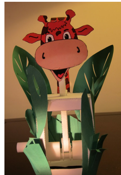
Figure 4. An automaton fabricated using a 3D printer and a computer-controlled die cutter.
