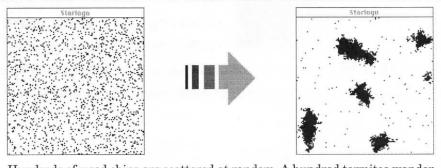
Hundreds of wood chips are scattered at random. A hundred termites wander around randomly, each following a set of simple rules: "If you're not carrying a chip pick up the next one you encounter. If you are carrying a chip, put it down near the next chip you run into. Then scoot away and repeat the process." After a while the chips are mostly in a few large piles although the rules the termites follow say nothing about building piles.
