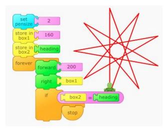
A clue: If you want to find an angle for the turn: with regular polygons their lines do not cross so their total turning is 360 degrees. Thus a regular polygon turns a total of 360 degrees. Notice the turtle makes external (not internal) turns.
