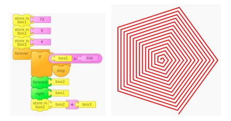
Notice: This stack has a different stop rule. The job is done when the forward step is greater than 300 or some other specific number.
